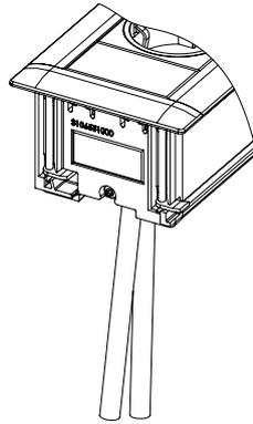
Fixed Power Supply Cable through the bottom of the profile
