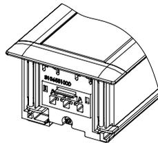
End cap with power input or output connector, depending on the surface thickness (max. 18 mm)
